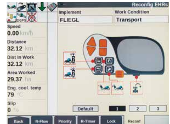
ISOBUS functions can be configured onto existing controllers such as the Multicontroller, joystick and control levers.
