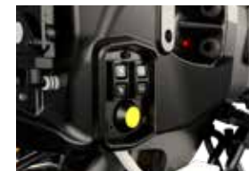
External controls are provided at the front and rear of the tractor for the hydraulic life, PTO and an additional control unit.
