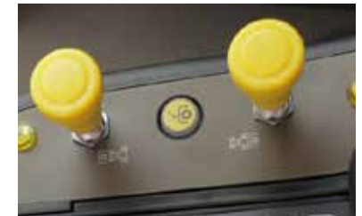
Electro-hydraulic activation of the rear and front PTO.
