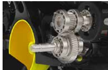
Direct power transfer from the motor to the front PTO.
